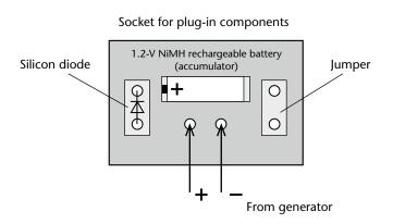
Make sure you are careful to get the polarity right when connecting the leads and plugging in the diode.
