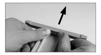
Keep the feet straight when pushing them off. The best way to remove the feet is to turn the rail upside down and use your thumbs to press the feet out of the rail (see the picture).
