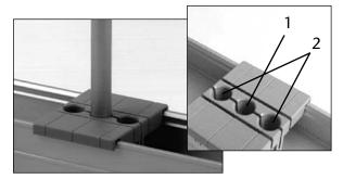
The clamp sliders can be attached to any position on the rail. They serve for insertion and fixing of the rods.
