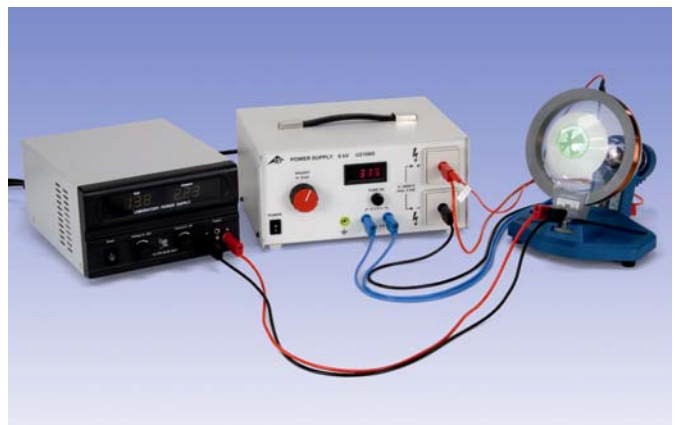
Fig. 3: Modified experiment set-up with an additional axial magnetic field
