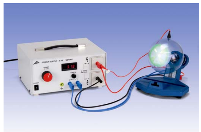
Fig. 2 Experiment set-up to demonstrate the straight-line propagation of electrons using a Maltese Cross tube
