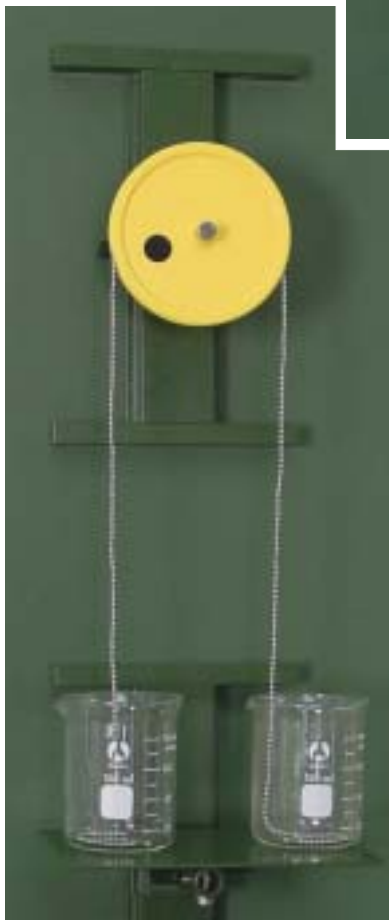
36 Experimental model of an angle lever
