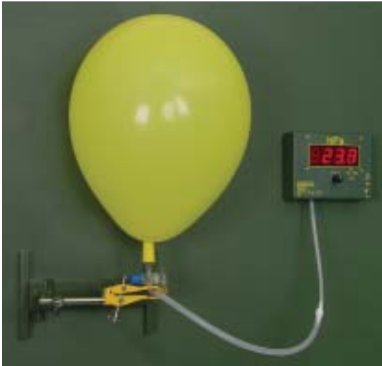
168 Measuring air pressure in a balloon
