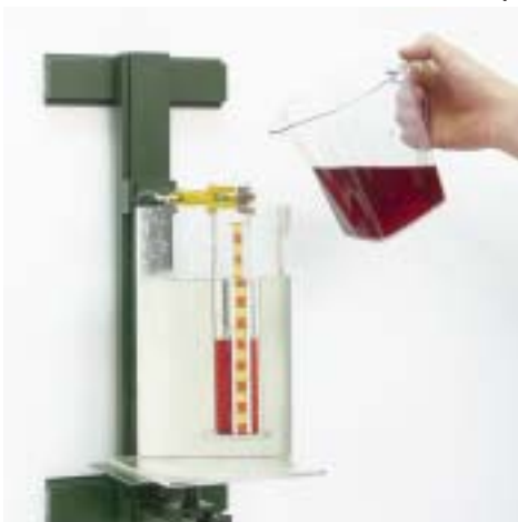
144 Measuring hydrostatic pressure using Hartl's apparatus
