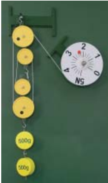
128 Block and tackle with four pulleys
