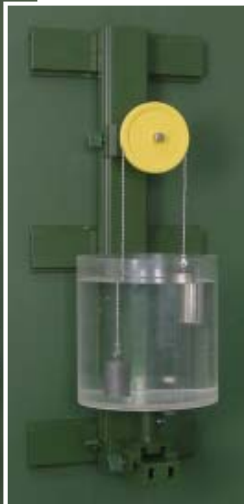
175 Buoyancy of bodies with different densities
