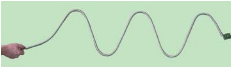
221 Standing waves with a fixed end
