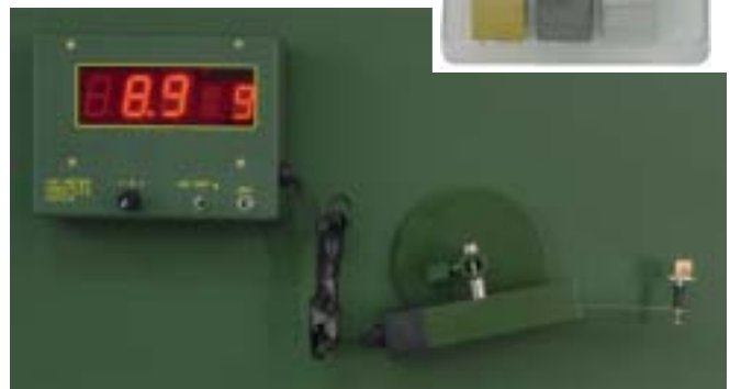
10 Measuring the density of solid bodies with the same mass
