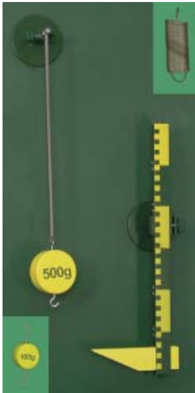
207 Determining the elasticity constant
