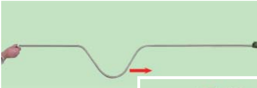
222 Wave reflection from a fixed end
