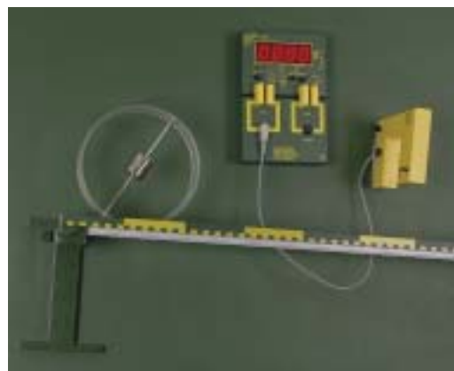
103 Centripetal force is dependent on mass, radius and angular velocity
