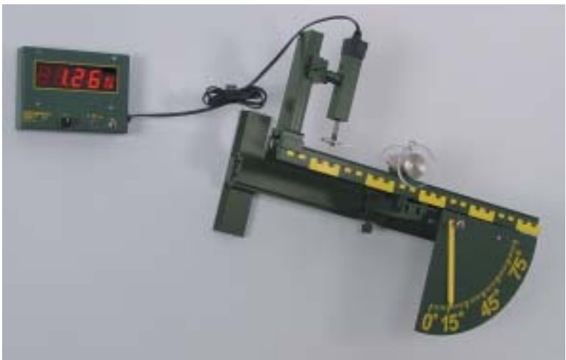
28 Force parallel to an incline
