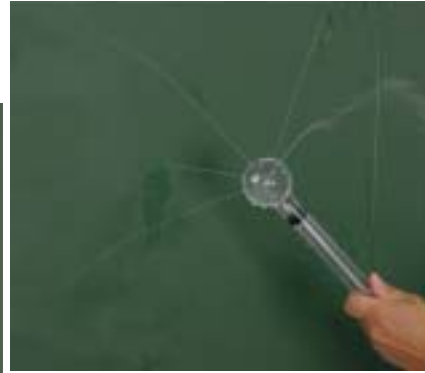
147 Distribution of pressure in liquids
