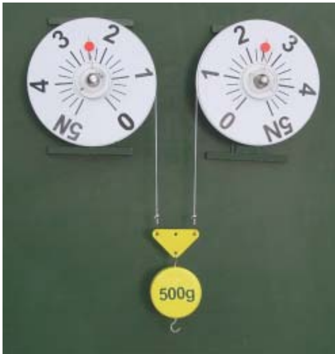
25 Composition of equidirectional forces
