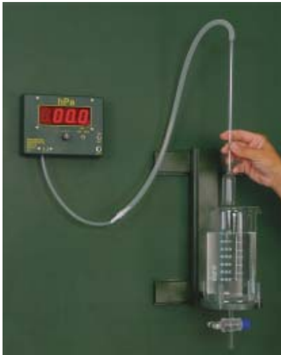
143 Measuring hydrostatic pressure using immersion sensors of different shapes
