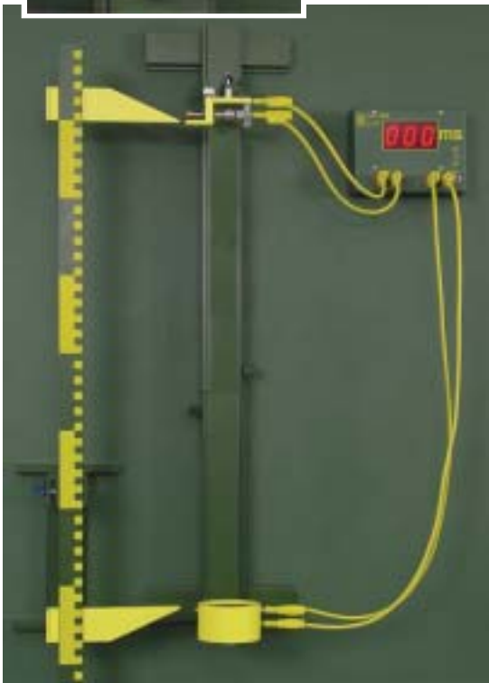
86 Free fall - measuring gravitational acceleration
