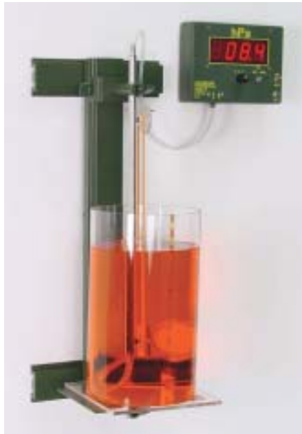
144 Measuring hydrostatic pressure using Hartl's apparatus
