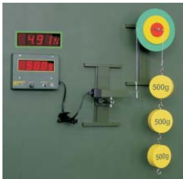
129 Parallel block and tackle with four pulleys
