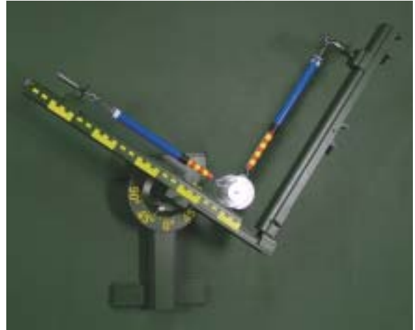
30 Force components on an incline
