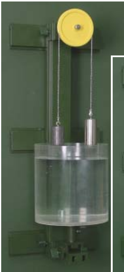
175 Buoyancy of bodies with different densities
