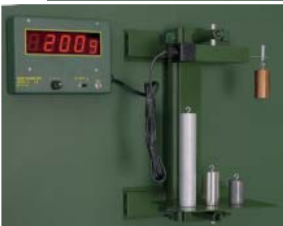
10 Measuring the density of solid bodies with the same mass
