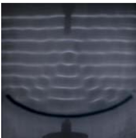
234 Reflection in a concave mirror
