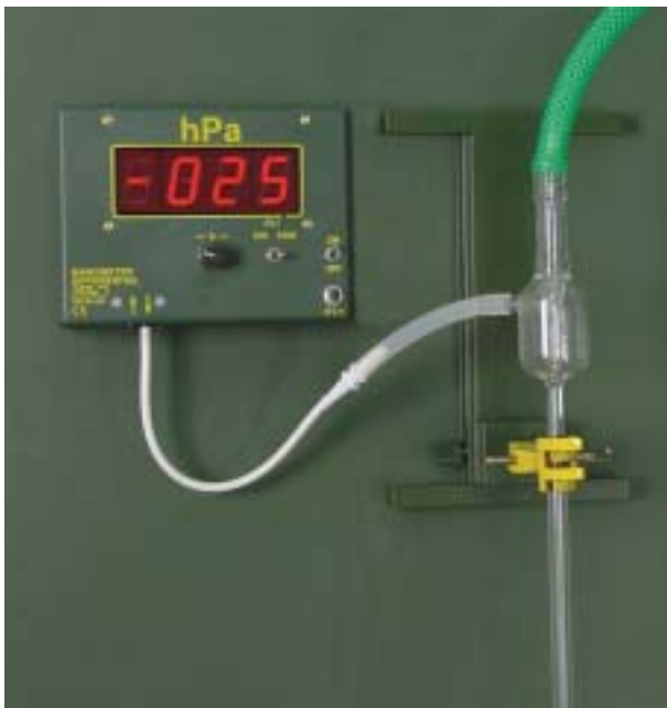
165 Measuring the vacuum in a water-jet pump
