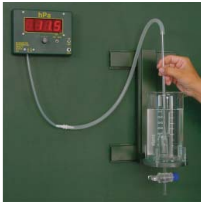
143 Measuring hydrostatic pressure using immersion sensors of different shapes
