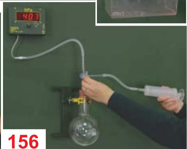
Measuring pressure change by density change
