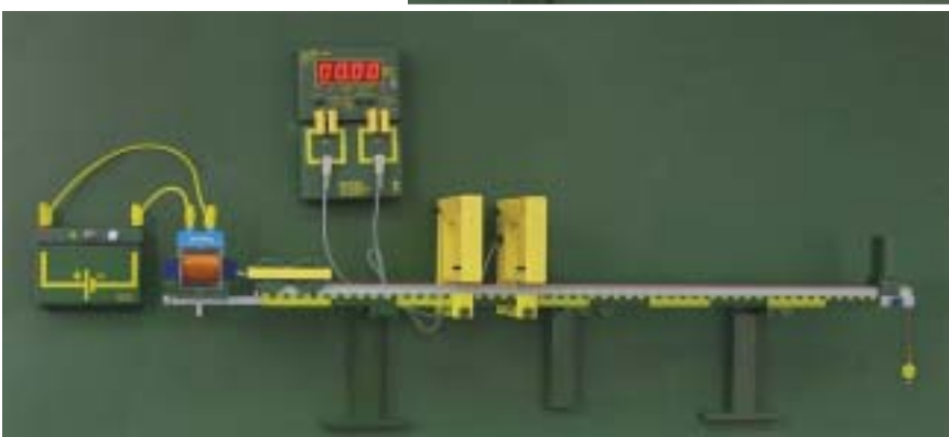
58 Law of time and acceleration applied to the accelerated uniform motion of a wagon
