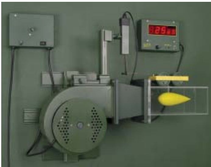
204 Air resistance and bodies' surface types
