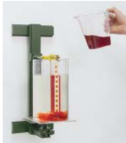
144 Measuring hydrostatic pressure using Hartl's apparatus
