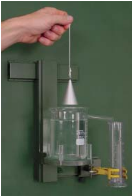
05 Measuring the volume of solid bodies by liquid displacement
