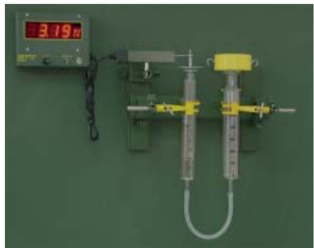
141 Pressure on different surfaces
