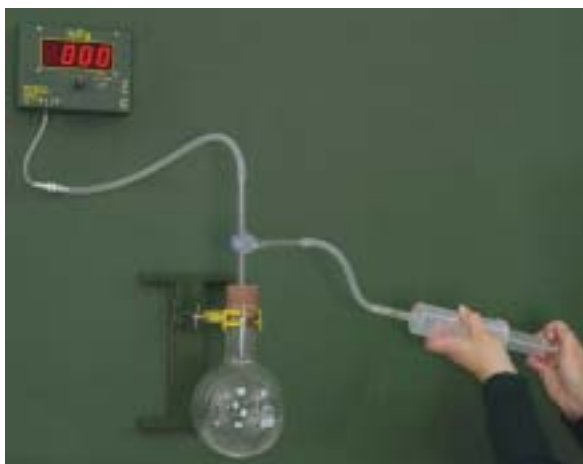
Measuring pressure change by density change
