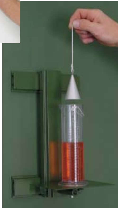
05 Measuring the volume of solid bodies by liquid displacement
