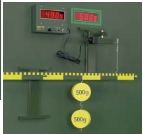
38 Position and force direction not relevant for a two-armed lever
