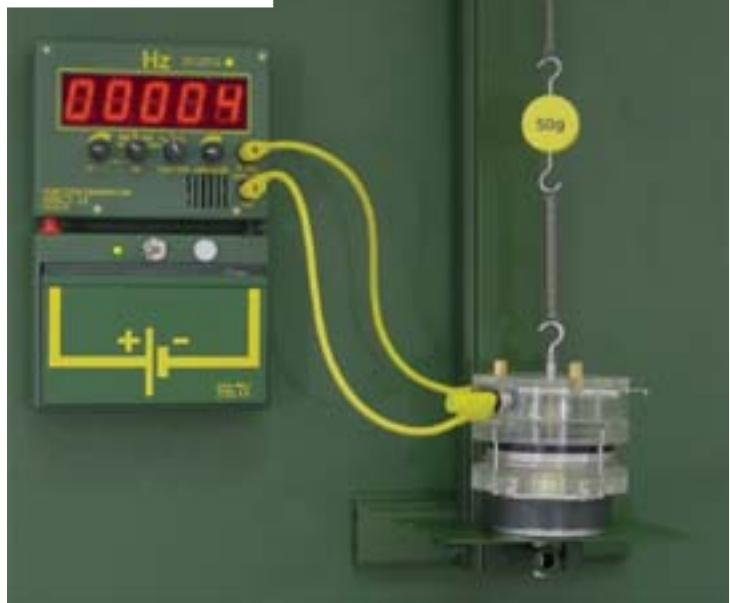
214 Moment of inertia and duration of torsional vibration
