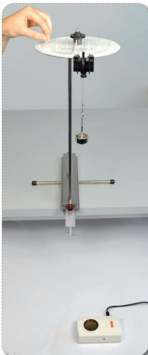
Demonstration of the law of angle and time in uniformly accelerated rotary motion
