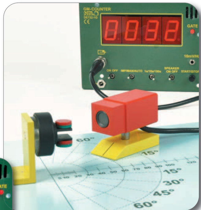
RAI 3.2 Behaviour of beta radiation in a magnetic field
