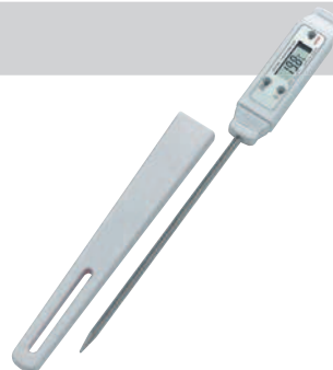
C4350-1A Thermometer SE, digital, 200 °C Digital precision thermometer, metal sensor, L = 125 mm, incl. protective cap; 6-mm LC display Measuring range: -40 ... +200 °C (-40 ... +392 °F); accuracy: \pm 1 °C; resolution: 0.1 °C Functions: hold, maximum and minimum temperature, battery-powered, automatic shutdown
