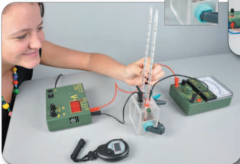
TDS 5.2 Thermoelectrical cooling, "Peltier effect"
