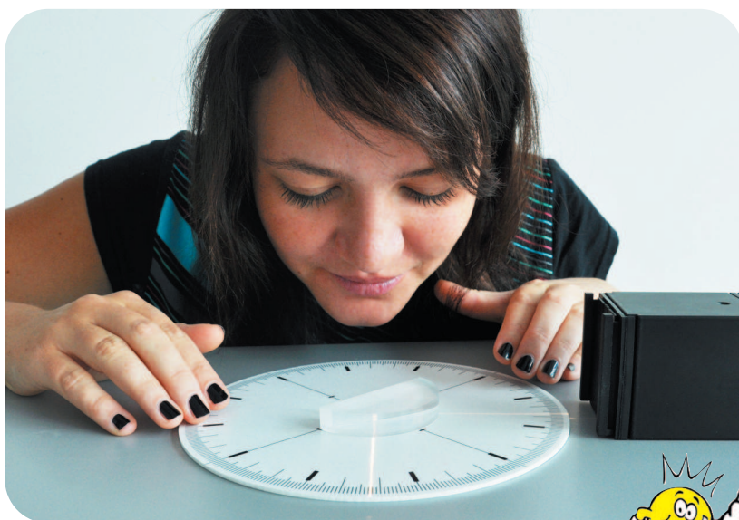
Optics set for experiments "on the desk" with halogen lamp 12 V / 20 W
