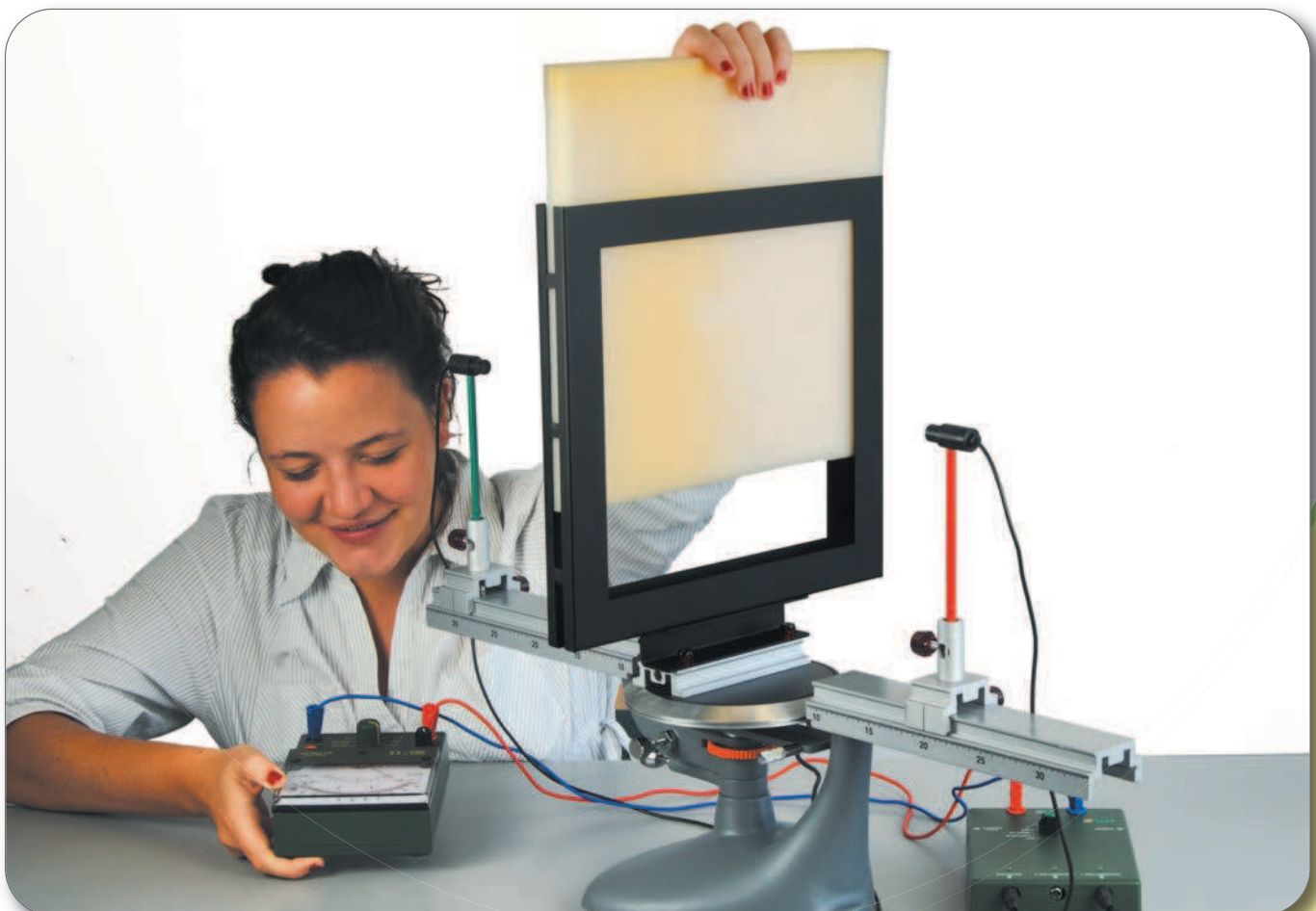
US 08 Absorption of sound waves by different materials
