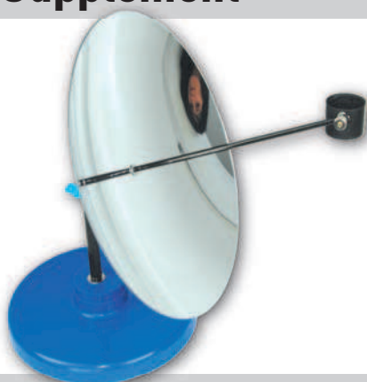
P2885-1P Parabolic mirror with stand High temperatures in the focal point of the mirror can be generated by bundling heat radiation; parabolic mirror made of plastic, small metal container mounted in the focal point for heating up various materials, large base plate and holder with adjustable pivot bearing for optimum setting of the angle of incidence.
